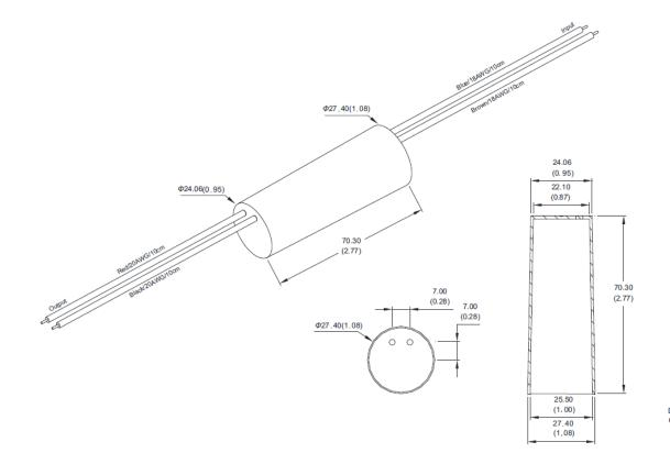
Dimensions mm (inch) Case Tolerance ±0.50 (±0.02)
